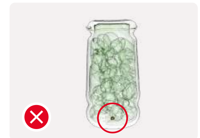
Non-compliant: Presence of a glass fragment
