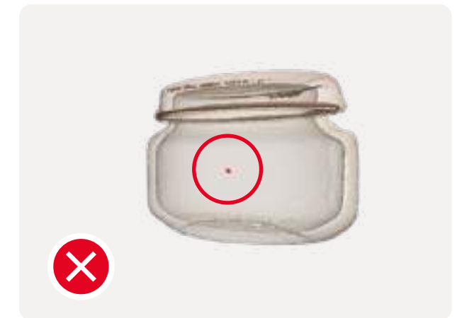
Non-compliant: Presence of a glass fragment
