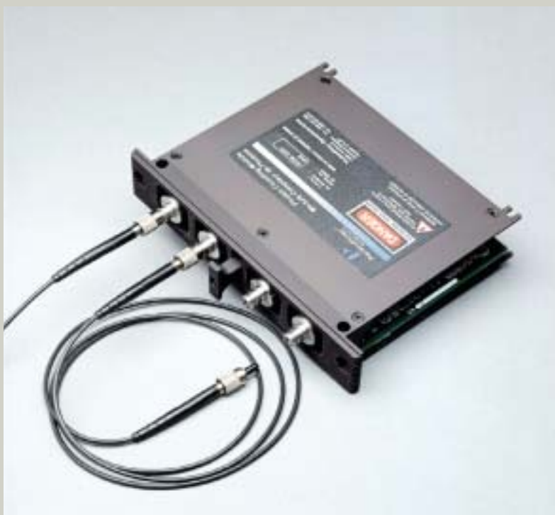
Figure 3. A new four-channel SPCM, which can be arrayed to provide cost effective and compact SPCM systems with as many as 100 possible channels.
